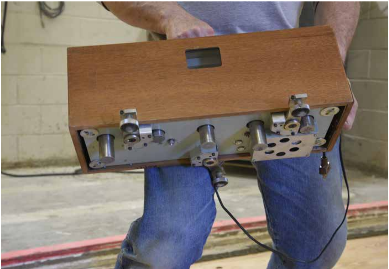
Above: calibrated impact sound generator used for IIC testing. Image Credit: Evan Schmidt, OSU TallWood Design Institute
